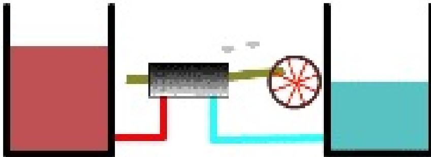
FIG. 1. A Carnot engine bridges a hot reservoir (left) and a cold reservoir(right)
